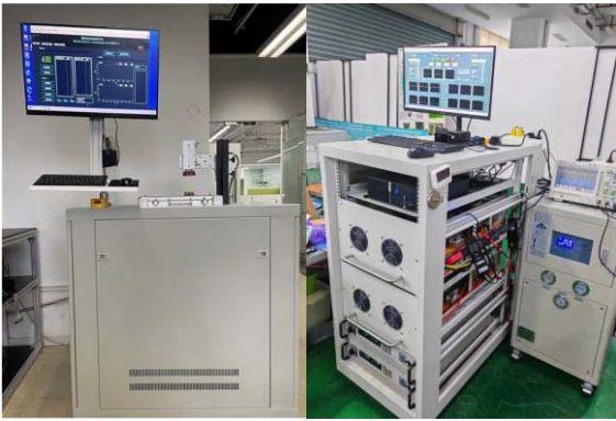
FIGURE 7. IGBT dynamic characteristics testing platform (left) and power cycling platform (right).
