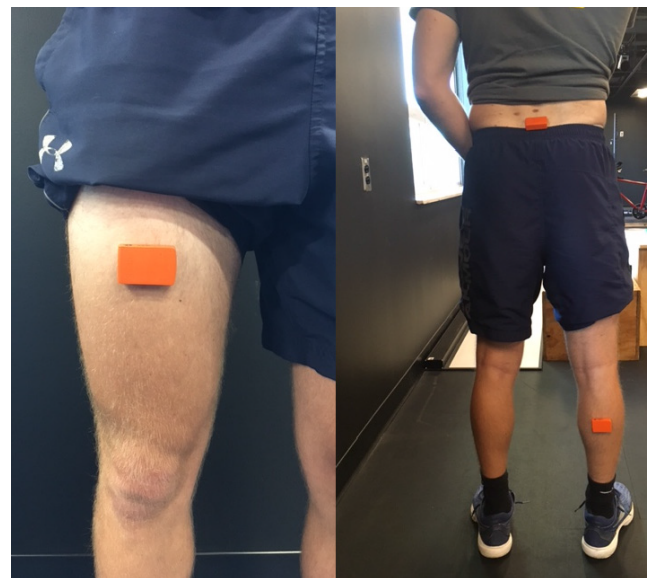
FIGURE 1. Motion sensors location and position for the IMU system.
