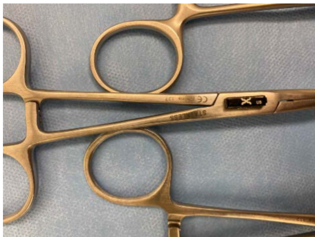
FIGURE 3. A Xerify Dash XS tag affixed to a hemostat via super glue.
