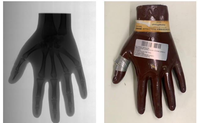
FIGURE 12. Victoreen Nuclear Associate Hand Phantom 76-634 x-ray image taken by SyncBox controlled TDI detector x-ray scanner. 0.5 mm aluminum filtration has been used. Exposure parameters are 60 kVp, 10 mA duration 1.8 sec. Total image acquisition time 5 seconds.
