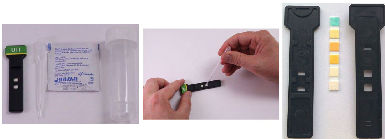
FIGURE 3. Disposable 'key' kit (left), sample being applied to lateral flow 'key' (center), and 'key' composite parts (right).
