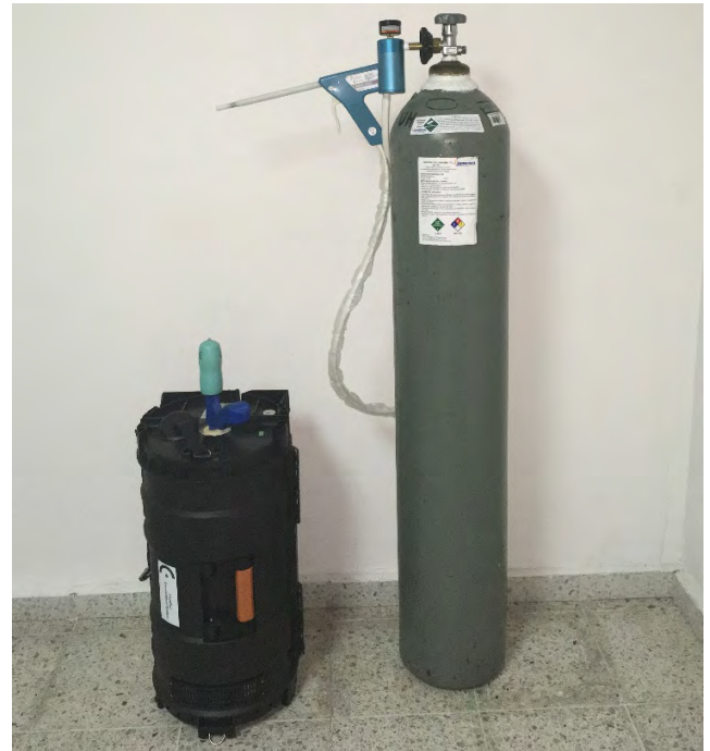
FIGURE 3. CryoPen (left) offers a smaller, gasless alternative to CO 2 -based systems for cryotherapy (right). CryoPen is also enclosed in a ruggedized container for easy transport.
