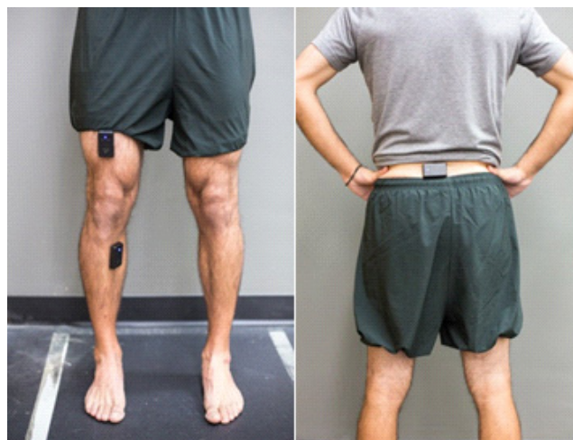
FIGURE 5. Sensor placement during SLS data collection.
