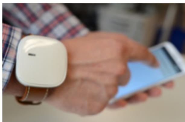
FIGURE 1. Sensor node equipped with the 3-axes accelerometer, gyroscope and magnetometer attached at the wrist together with the data acquisition device (smart phone).
