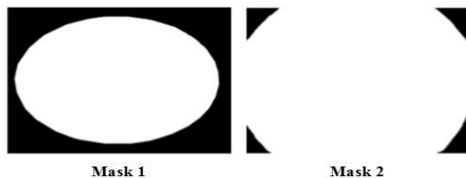
FIGURE 5. Mask 1 and Mask 2, used in the segmentation algorithm to prepare the image for the initial state of the active contour and to remove the corners.
