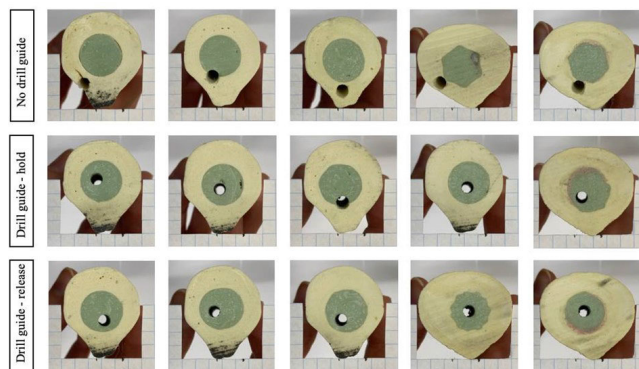
FIGURE 11. Drill hole locations at the cement plug exit point separated for the tree different conditions.
