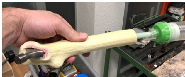
FIGURE 7. Bone model, cement and hip implant preparation. The cement is injected in the bone cavity via a syringe.
