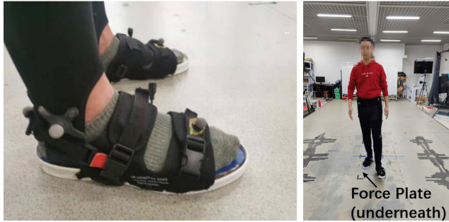
FIGURE 8. A participant wearing the instrumented shoe system and the overview of the experiment set-up.
