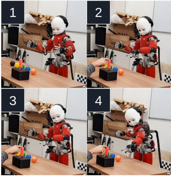
Fig. 3. Uncertain movement's steps: (1) the rest position, from which all the robot movements began; (2) the thoughtful movement; (3) the final gaze; (4) the pointing action.
