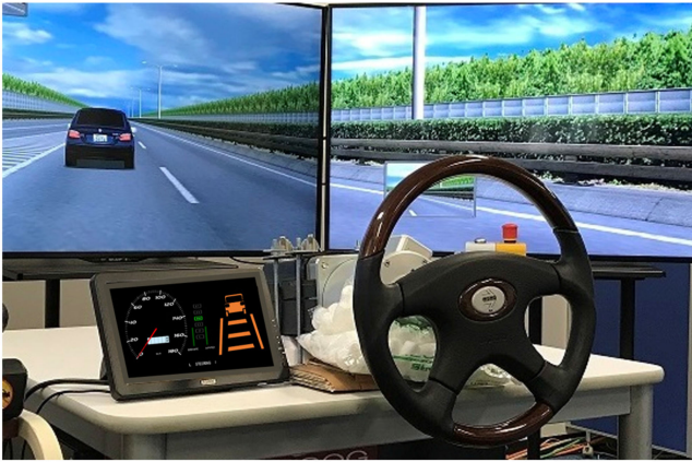
Fig. 2. Fixed-base driving simulator operated by a R&D driving simulation system and electric control loading systems.
