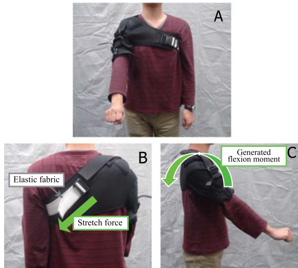
Fig. 1. SEnS. Elastic fabric generates the shoulder flexion moment shown as the arrows. One side of the elastic fabric is fixed at wearer's breast by a harness wrapping around the breast. (a) Front view. (b) Back view. (c) Side view.
