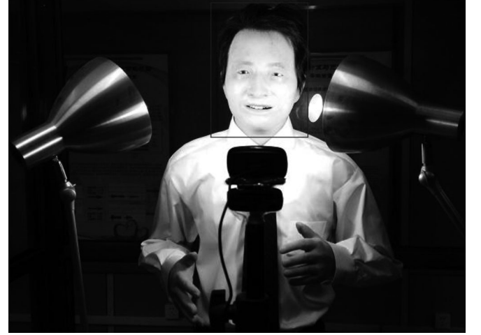
Fig. 3. Experimental setup used for data collection for solving forward kinematics model.
