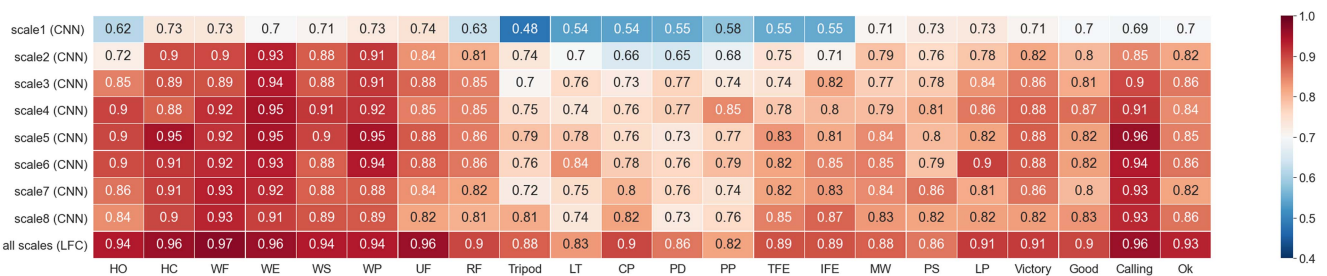
Fig. 12. Heatmap of results (f1-score) for gesture recognition using different scale representation from CNN and LFC. The vertical axis represents different scale representation (scale1 ~ scale8) from different layers' results of CNN. Results of all scales using LFC are shown in the bottom for comparison.
