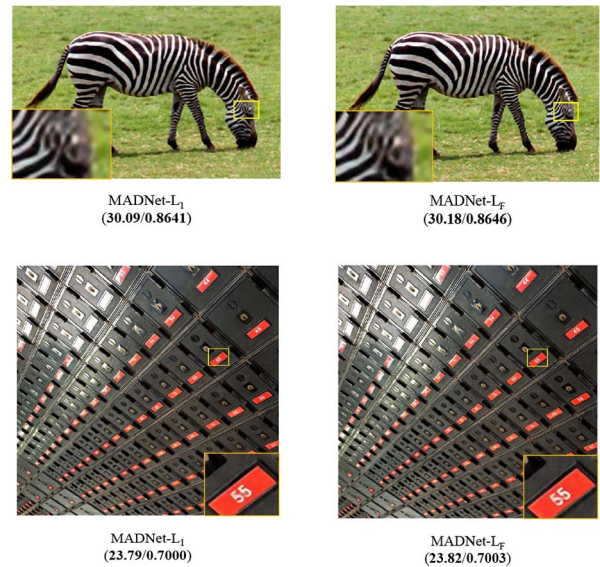
Fig. 7. Comparisons of the loss function for \times 3 SR. On the top row, the “zebra” image from the Set14 dataset, the image processed with L_F has clear details in the area around the eye. On the bottom row, the “img006” image from the Urban100 benchmark, the L_F method super resolves the number “55” sharply.
