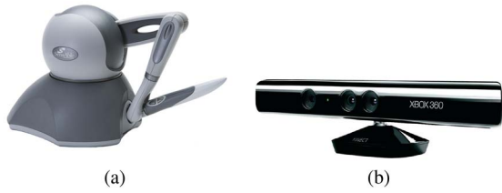
Fig. 3. Devices used in the teleoperation system. (a) Omni joystick. [Captured from: http://www.geomagic.com/ ]. (b) Kinect sensor. [Captured from: http://www.microsoft.com/ ].
