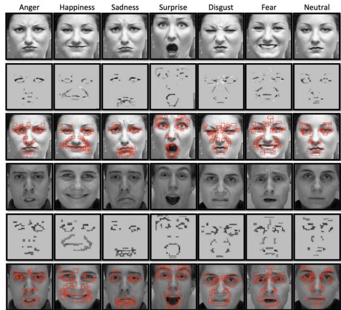
Fig. 4. Selected optimal features and their distribution for each expression using the proposed mGA-embedded PSO algorithm (rows 1–3: CK+ images and rows 4–6: MMI images).
