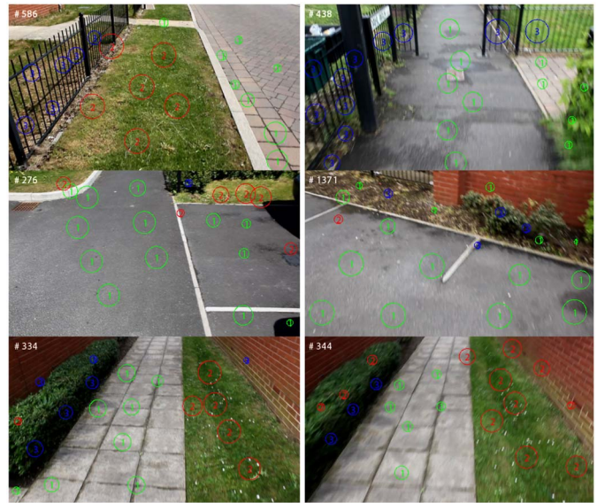
Fig. 16. Subjective results. Label 1 (green), label 2 (red), and label 3 (blue) correspond to the areas classified as hard surfaces, soft surfaces, and unwalkable areas, respectively. The size of the circle indicates probabilities—bigger implies higher confidence of classification. The left and right columns are from sharp and blurred frames, respectively. Classification accuracy (top to bottom) of left column: 87.07%, 89.96%, and 86.79%; right column: 79.75%, 67.32%, and 75.17%.
