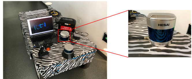
Fig. 4. Experimental vehicle is equipped with a 64-line Hesai LIDAR.
