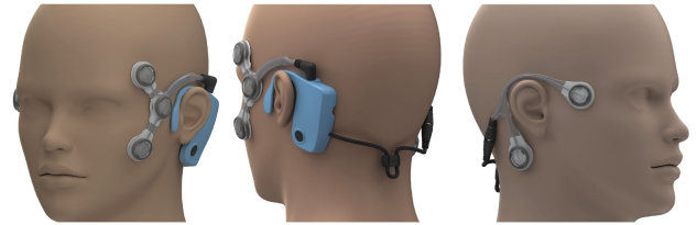
Fig. 1. The CAVA device consists of five electrode pads contained within two, detachable mounts, and an electronic logging unit which sits behind the left ear. Two electrodes placed near the temples on either side of the face capture horizontal eye movement. Two electrodes above and below the left eye record vertical eye movement. A fifth electrode beneath the right ear provides a reference voltage. The device also contains a push button for patients to log events of interest, such as the onset of an attack of dizziness.
