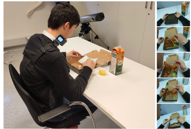
Fig. 1. A subject wears a GoPro Hero 7 Black camera, which records the entire eating episode in a passive way. The camera is mounted on the shoulder at the same side as the subject's dominant hand. This position provides the camera with a good view that can capture both the mouth and dominant hand, which facilitates bite counting and consumed food item recognition from the recorded egocentric video.
