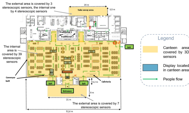
Fig. 7. 2D map of the canteen with an indication of the position of sensors and monitors installed in external and internal areas.
