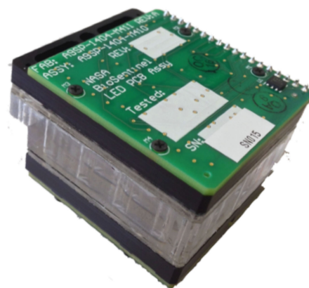
Figure 11. Growth curves ( top ) recorded using spaceflight optical/fluidic/thermal prototype shown ( bottom ) for wild-type S. cerevisiae with added aB (filled symbols) and cell-free control microwells (open symbols); LED wavelengths as indicated.
