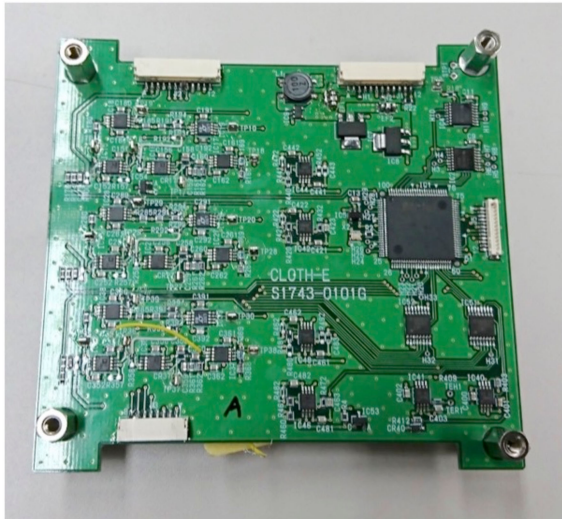
Figure 7. Electronics board of CLOTH (Engineering Model).
