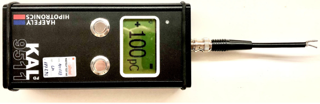
Fig. 9. PD calibrator with adapter cable for connection to the MV cable. R_{t1} can be soldered between the separated conductors if necessary. The oscilloscope was connected in a similar way, with optional R'_{t2} .
