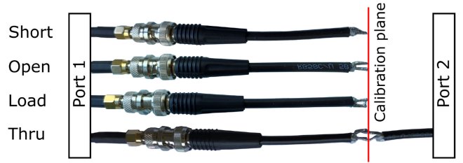
Fig. 5. Adapter between VNA and MV cable and corresponding calibration scheme.
