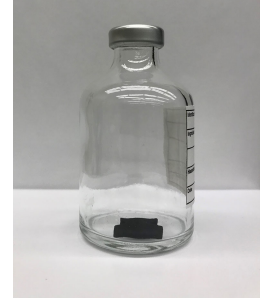
Fig. 8. EPDM elastomer sample tested for compatibility with C 3 F 7 CN gas.
