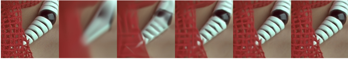
Fig. 5. An example of mean estimated reconstructions of a 128 \times 128 image. Original (left) followed by models with 25, 100, 250, 750, and 2000 components, i.e. ranging from 1 kernel covering \pm 655 to \pm 8 pixels on average. It is clear that SMoE provides a continuously-refined low-pass version of the original.
