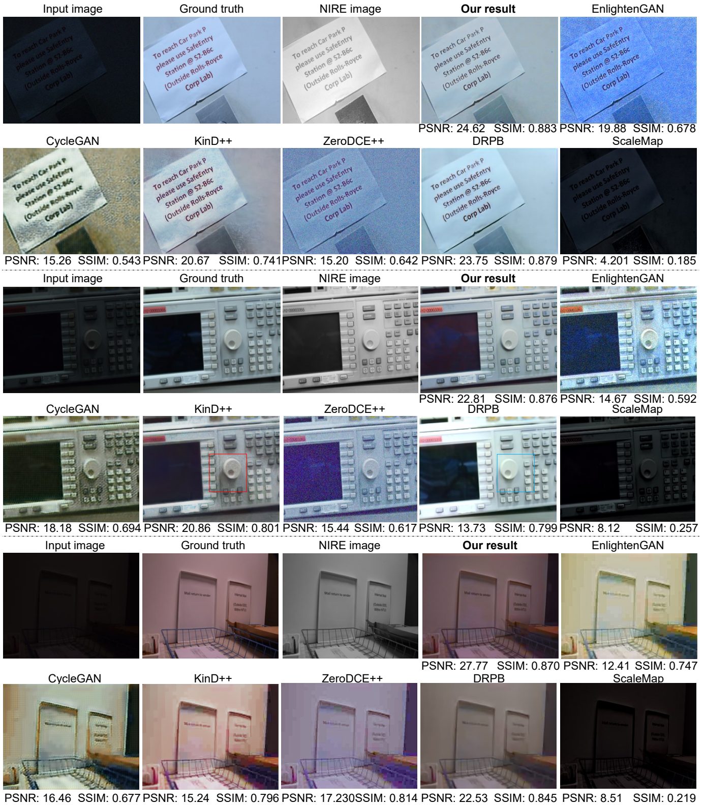
Figure 9: Three examples captured by the digital cameras with result obtained by our method, EnlightenGAN [31], CycleGAN [30], KinD++ [21], ZeroDCE++ [23], DRPB [52], and ScaleMap [16]. The SSIM and PSNR values are shown below each image. The red and blue boxes denote the regions with over-smooth effects and other artifacts.
