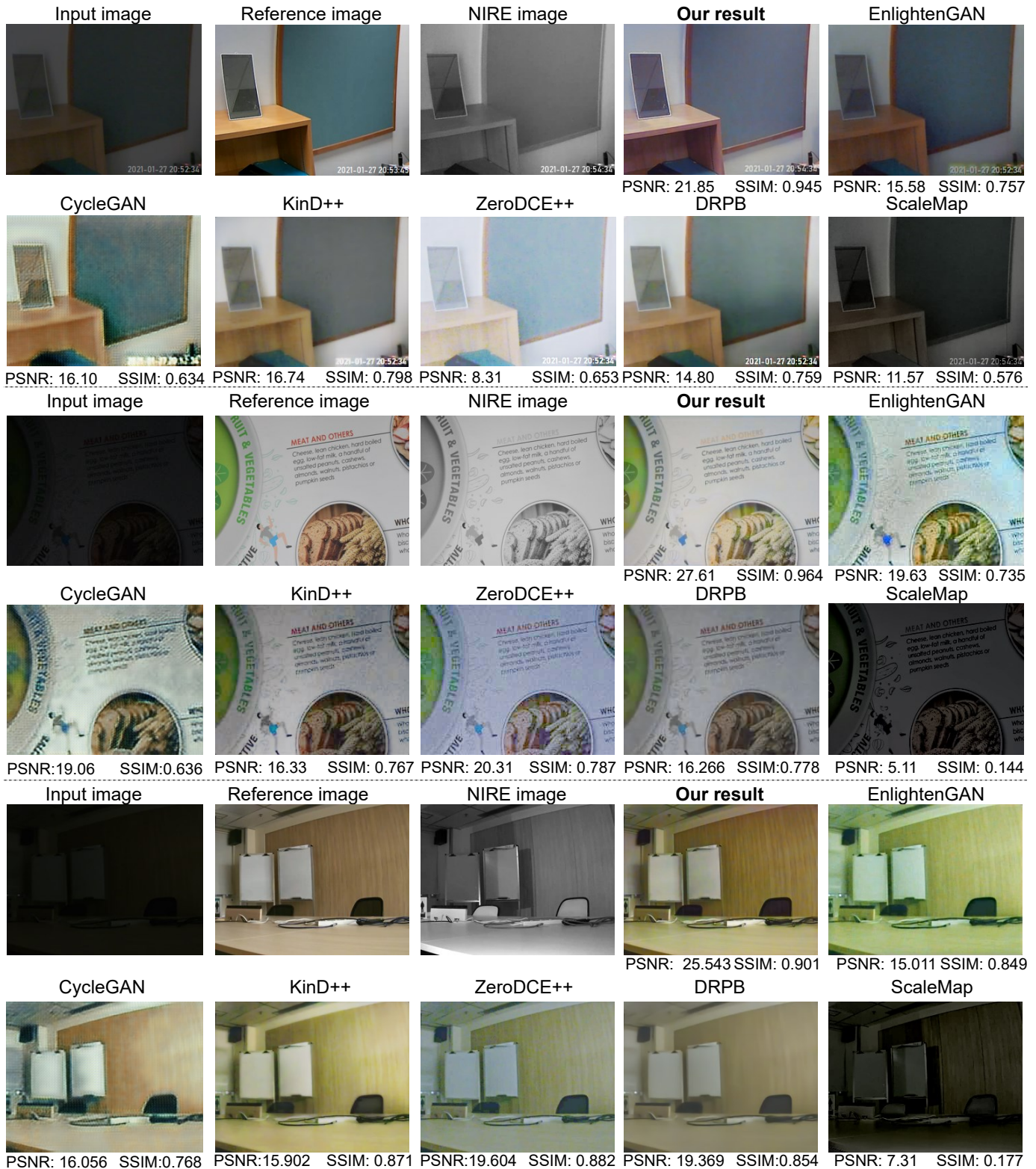
Figure 10: Three examples recorded by the surveillance cameras with results obtained by our method, EnlightenGAN [31], CycleGAN [30], KinD++ [29], ZeroDCE++ [23], DRPB [52], and ScaleMap [16]. The SSIM and PSNR values are shown below each image.
