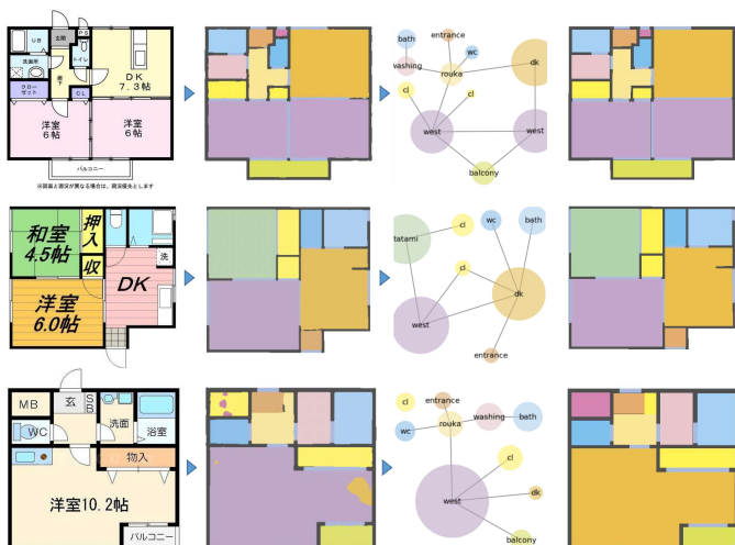
Fig. 5. Examples of input images (first column on the left), inferred semantically segmented images (second column), extracted graphs (third column), and grand truth segmented images (forth column).
