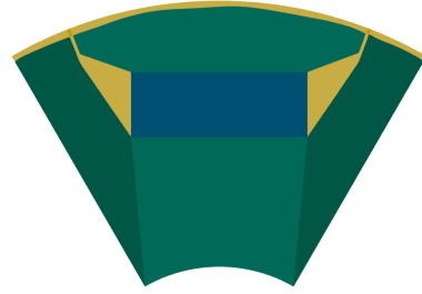
Fig. 12. Results of shape optimization (8)–(9) under full load condition. The shape of the rotor was optimized, minimizing the total harmonic distortion with the physical constraint (29) maintaining the average torque. Shape and position of the permanent magnet was fixed.
