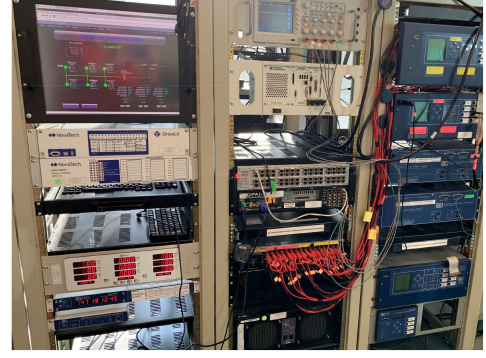
Fig. 6. OPAL-RT platform HIL setup of NSPS.
