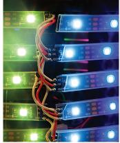
THE GREAT PRETENDER: An Arduino Leonardo [above] acts as a USB device mimicking a MIDI-enabled electronic instrument. It converts received notes into colors displayed on a strip of LEDs [right].
