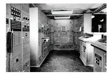
**DIVIDE AND CONQUER:** The complete SIGSALY voice scrambler was a huge machine [bottom] that relied on many analog-to-digital converters. The heart of the converter was a resister divider ladder [top photo and schematic, middle] connected to thyratrons. In my re-creation, I have added neon indicator lights.
