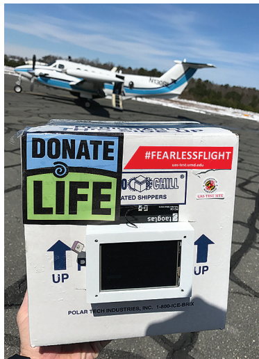
PRECIOUS CARGO: Researchers measured whether a kidney, stowed in a cooler, could be delivered safely by drone. A custom sensor inside the cooler monitored the temperature and vibration of the organ during its trip.
