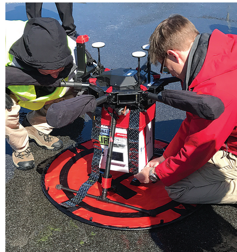
PRECIOUS CARGO: Researchers measured whether a kidney, stowed in a cooler, could be delivered safely by drone. A custom sensor inside the cooler monitored the temperature and vibration of the organ during its trip.
