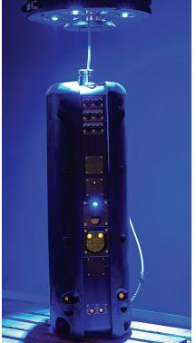
**EXTERMINATE!** The Stingray bot [above] is attached to a buoy and lowered into a fish pen [top left]. The bot's image sensors and software scan for lice attached to nearby salmon. If they spot one, the bot lets rip with a 530-nanometer (green) laser [bottom left].
