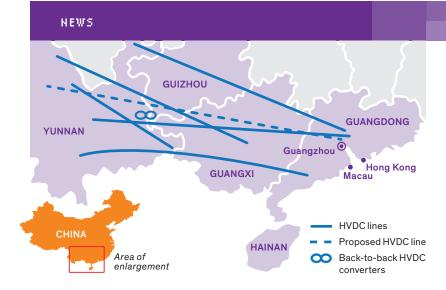
advances in solid-state power electronics. Solid-state conversion between AC and DC has enabled high-voltage direct current (HVDC) transmission lines that move electricity farther and more efficiently than AC lines. And, when paired, "back-to-back" DC converters allow the electrical exchange of power between nonsynchronized AC grids.
