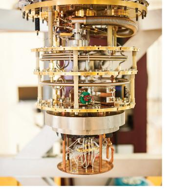
**COOL QUANTUM TECH:** This dilution refrigerator can cool quantum dots to less than 5 millikelvins for experiments in quantum computing. New quantum algorithms could allow quantum computers to process data at a much higher speed, allow-
