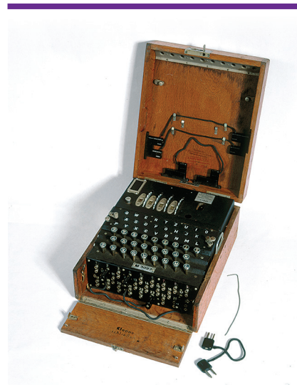
A WAR MACHINE: This Enigma can be identified as once belonging to the German navy, as it uses four encoding rotors—army Enigmas had only three.
