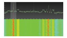
WATCHING RADIO: This screenshot from Gqrx shows two FM stations. The central spikes are the analog stereo broadcast, while the squared-off signals on either side are digital radio transmissions. You can tune in and listen to a station by clicking on its center frequency. The gray stripe indicates the bandwidth of the user-selected software demodulator.
