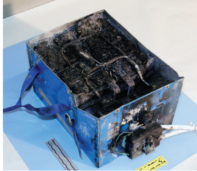
BURN OUT: Thermal runaway cooked this battery from an auxiliary power unit in a Japan Airlines 787.
