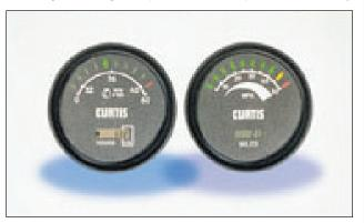
Both the tachometer and speedometer from Curtis Instruments Inc. employ multicolored light-emitting diodes to display speed on a segmented analog scale and to highlight critical portions of the speed range. The tachometer's integral numeric display records engine-use time; the one in the speedometer is an odometer.
