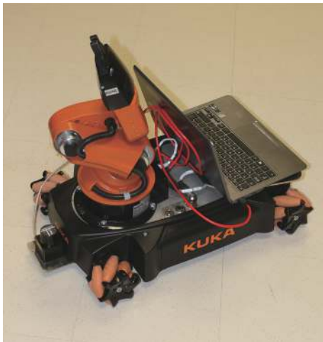
Fig. 3 KUKA youBot equipped with a 2-D LiDAR and on-board laptop
