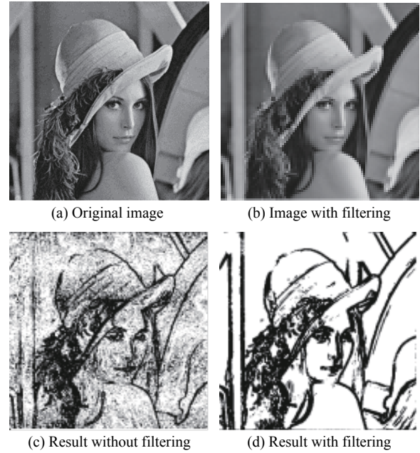
Fig. 5 Comparison of the edge detection quality with and without filtering conditions
