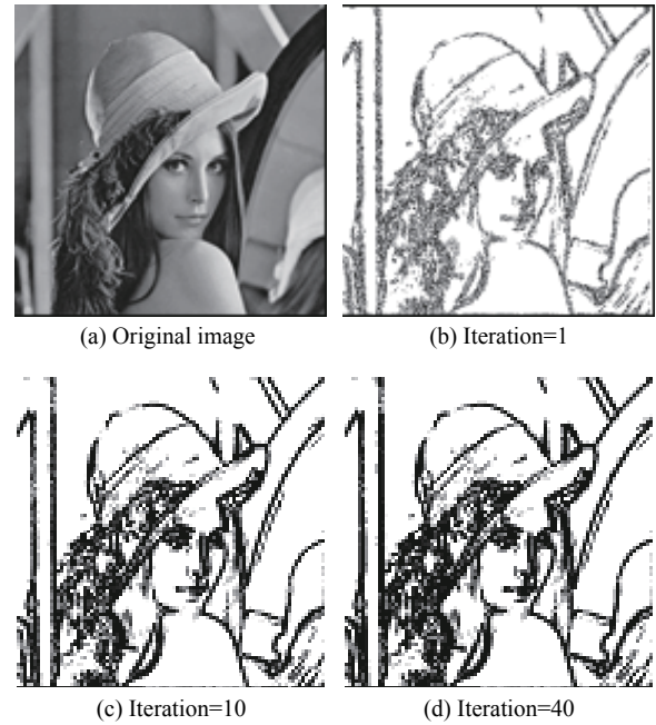
Fig. 3 Comparison of the quality of the edges detected from the Lena image
