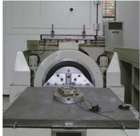
Fig. 10 Acceleration response experiment for 1 g sinusoidal vibration input
