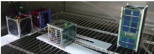
Fig. 8 EM-II of FloripaSat-I prepared for thermal cycling (center)
