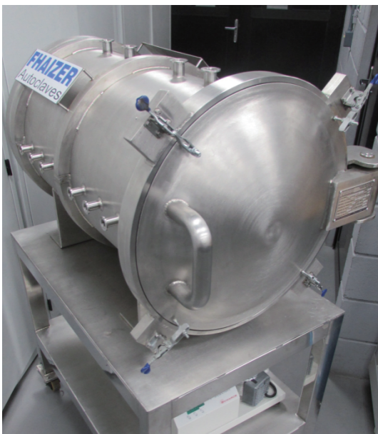
Fig. 17 Thermal vacuum chamber for preliminary out-gassing tests
