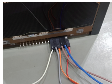
Fig. 18 Umbilical pins for communication, software programming and recharge of batteries
