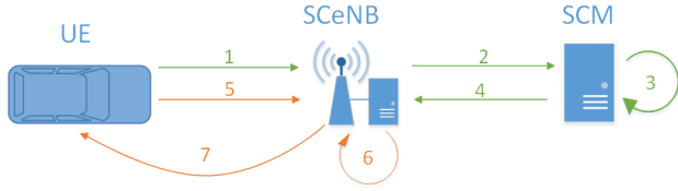
Fig. 2 Illustration of the interactive process, where the green line represents the transmission of the information of the request, and orange line represents the transmit of the data of the request data.
