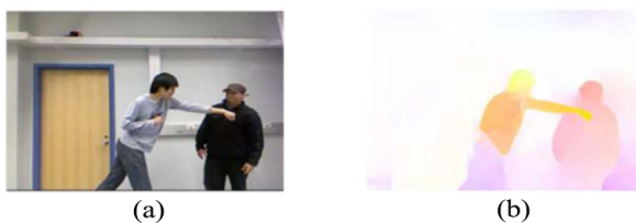
Fig. 5 Characteristic representation of the optical flow field [61] . (a) Real human action sequence; (b) optical flow.
