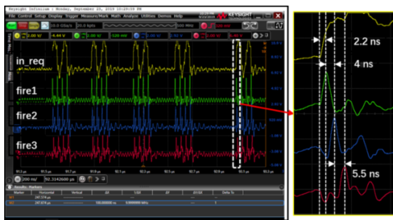
Fig. 13 Test results of the asynchronous CNN accelerator test chip.
